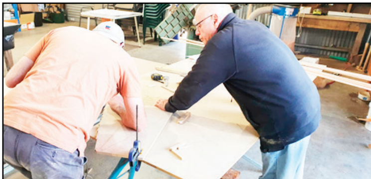
Kevin & Murray in the process of lofting the plans onto the moulds
