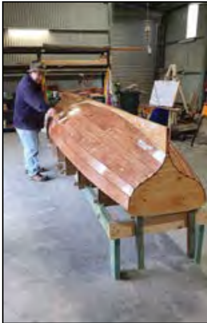
A coat of resin being applied
