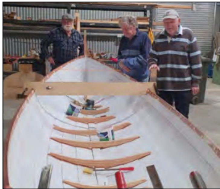
Fitting of the Ribs
